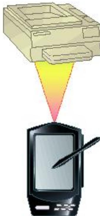
Fig. 2 . IrDA communication between a PDA and a printer (point to point)
